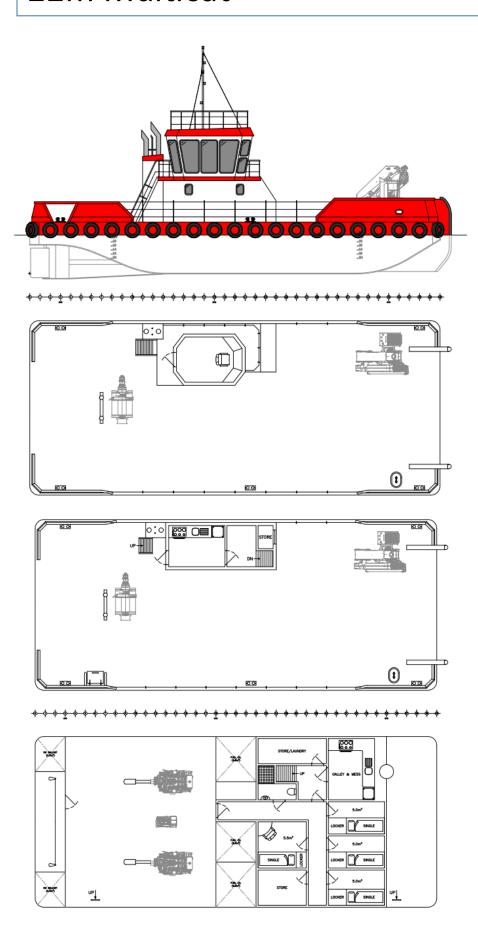
Length Hull22.55 mLength Waterline21.80 mLength Overall22.55 mBeam Hull8.50 mDraft2.14 m
